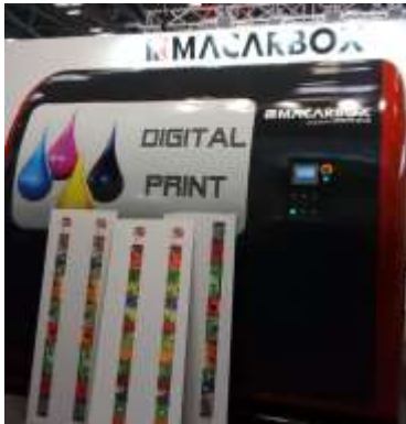
Macorbox – prototype 360 x 360 dpi – AQ or oil based inks
