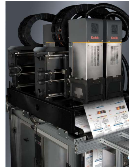
Kodak S Series Prosper heads - 7 colours 200m/min concept press with Uteco film transport – aqueous inks with primer
