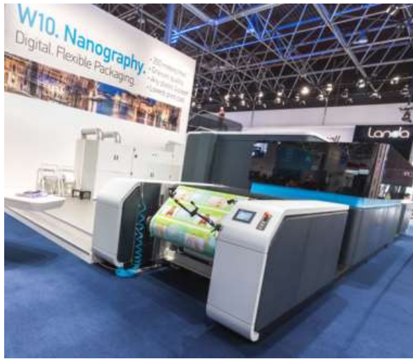
Landa W10 Fujifilm Samba print heads Aqueous inks
