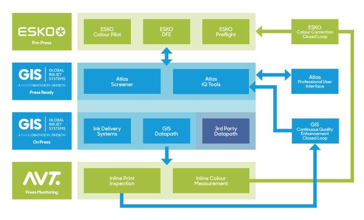
GIS offers the Esko DFE as an integrated component with GIS Atlas software. GIS supplies a pre-integrated linked Esko solution so that users have a complete, end-to-end workflow with system control to optimise and maintain print quality.
